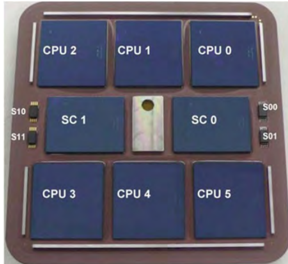
Figure 5: IBM z-microprocess using MCM technology with ceramic interposer.
