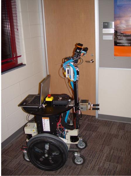
Figure 72: The Segway RMP 200 with LMS 291 laser scanner for wall measurements and a Prosilica 650c camera with a Hokuyo UTM30 laser scanner on a PTU-46-70 pan-tilt unit. Four caster wheels were added for stability. The robot is shown in a position typical of reading a door sign.
