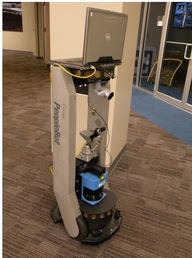
Figure 37: The robot platform used for these experiments. The camera attached to the laptop is the one that is used to detect the AR ToolKit Plus markers.
