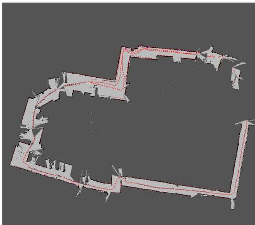
Figure 80: The robot has proceeded further along and it has just re-observed a door sign from the first time around this loop. The map is corrected and the robot now knows where it is.
