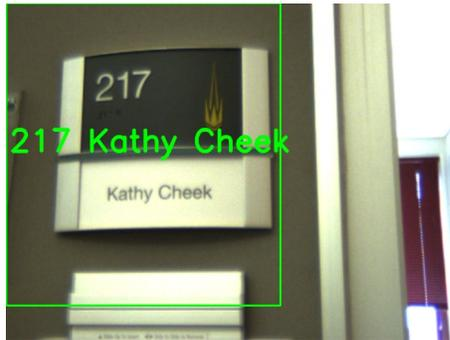
Figure 73: This sign is recognized and a measurement is made in the mapper. Google-Goggles has read both the room number and the text, so this sign can be used for data association.
