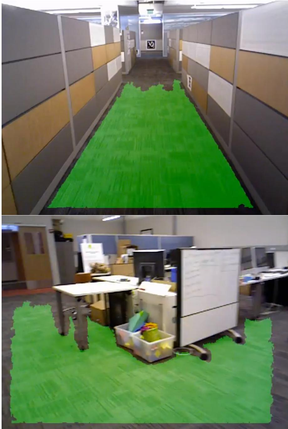
Figure 24: Example scenes of Kinect data segmented using our approach. This was performed to validate the segmentation approach during the development of the stereo tools.
