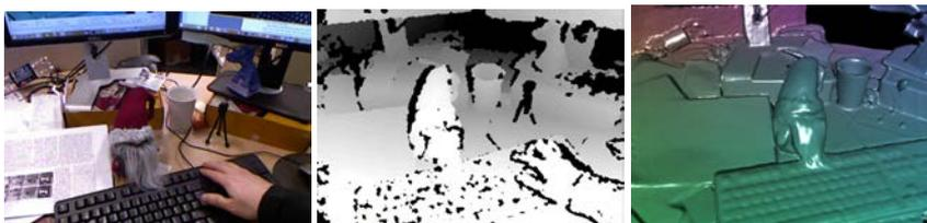
**Fig 17. Sample KinectFusion results. Left: color image from Kinect. Middle: a single depth map from Kinect. Right: reconstructed surface using KinectFusion (Newcombe *et al.* 2011a).**
