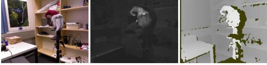
**Fig 7. Sample Kinect images from a scene. From left to right: color, infrared, and depth.**
