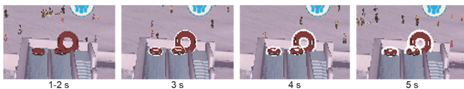
Fig. 8. An animated pulsating glow effect on an interactive object, e.g., rings in the center of the images, within a 3D VE. The size of the effect varies from 0 to 4 pixels within a 5-second timeframe.
