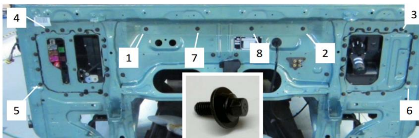
Fig. 11. The sequence in which the first 8 screws are fastened.
