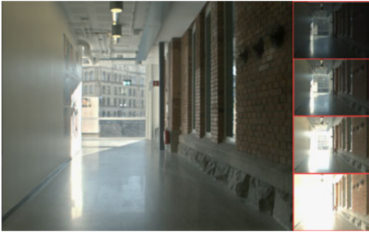
Figure 5.11: Left: A full resolution locally tonemapped frame from a video sequence captured with the HDR video camera. The image is reconstructed from four 4 Mpixel sensors at 26 fps. Right: Four gamma mapped images 2 f-stops apart from the same HDR-image.
