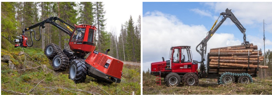
Figure 1: Harvester and Forwarder (Lahtinen, 2011)
