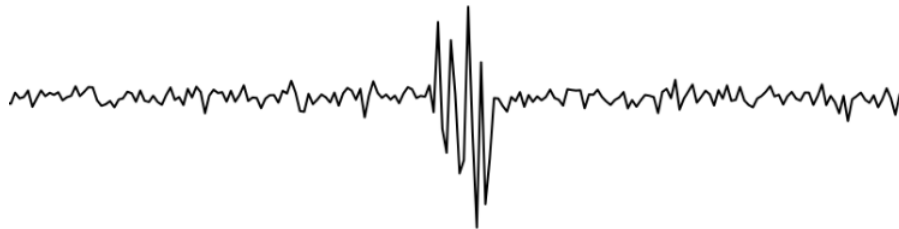
Figure 1.1: A real-valued discrete time series with a subsequence in the middle that shows tendency of being anomalous.
