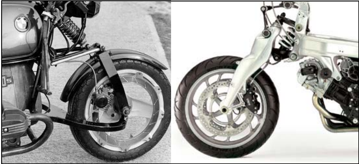
Figure 3.10. Foale/Parker front suspension design to the left with a single sided lower swing arm and extended upright connected to a triangulated upper wishbone taking normal loads (Foale, 2002). Duolever or Hossack et al. design to the right (Rider Magazine, 2005).
