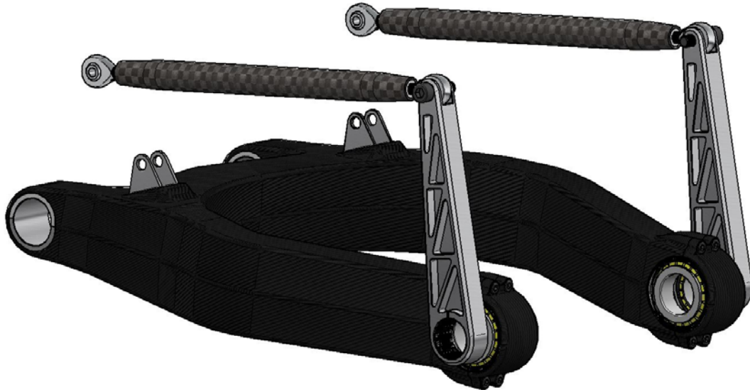
Figure 8.13. The suspension linkage, consisting of a swing arm, torque arms and torque struts. The torque arms are mounted to the transverse axle which is excluded from the figure why they appear to be floating in mid air.
