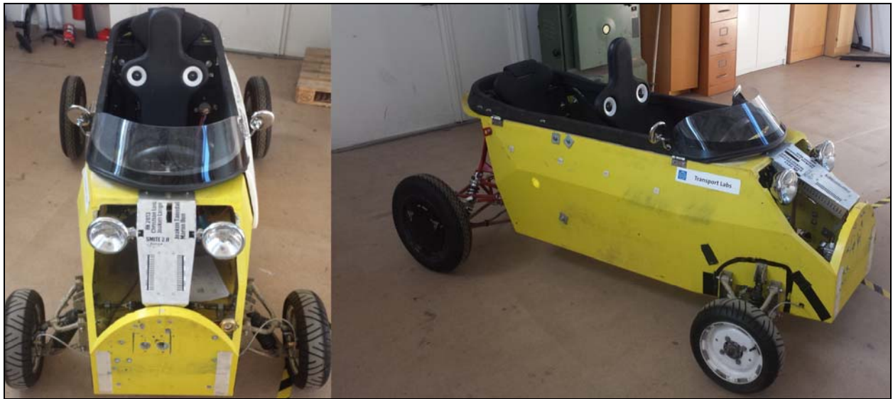
Figure 4.4. The small two-seated electric vehicle called Electra in the lab hall of ITRL.
