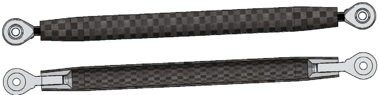
Figure 8.15. The composite torque strut, the threaded inserts are tapered and adhesively bonded to the tube.
