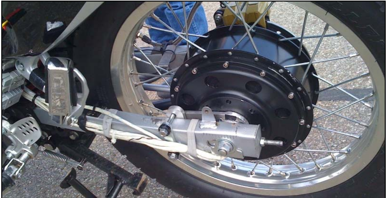
Figure 3.16. A common type of motorcycle hub motor with spoke attachment (Electricbike, 2014).
