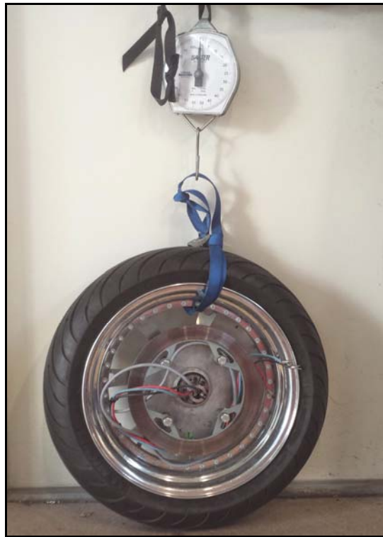
Figure 5.8. Weighing the wheel assembly used for friction coefficient measurement (resting on ground).
