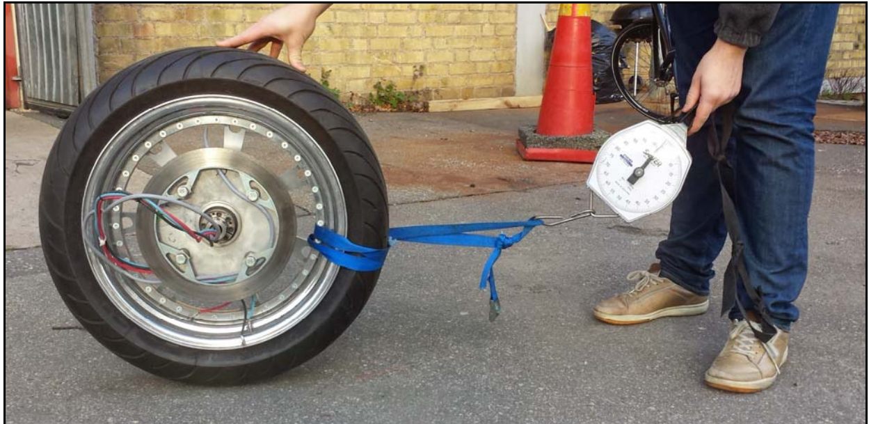
Figure 5.9. The setup for measuring tire friction coefficient, during measuring wheel rotation is constrained.
