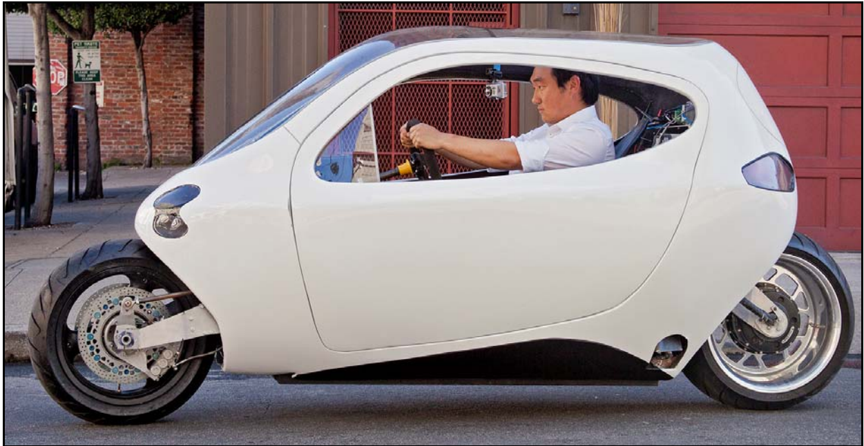
Figure 3.15. The Lit Motors first prototype with front swing arm, hub steering and rear wheel electric hub motor (Lit Motors, 2012)
