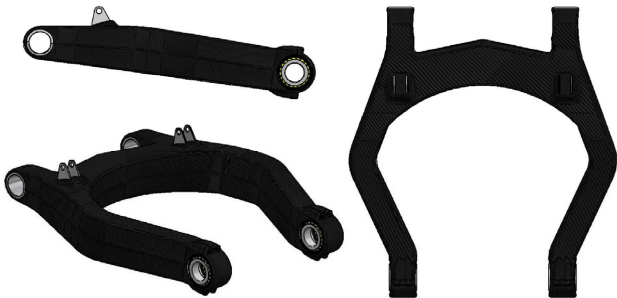
Figure 8.14. The composite swing arm from different viewing angles.
