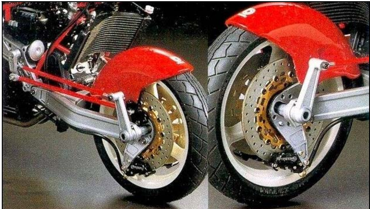
Figure 3.13. The Bimota Tesi with hub centre steering and struts fixed to torque arms mounted to the transverse axis (SportbikeRider, 2012).
