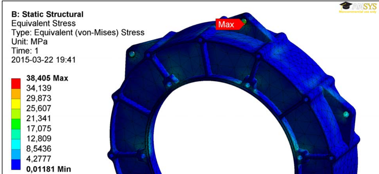
Figure A-III.7. The converged stress field for the motor cover.
