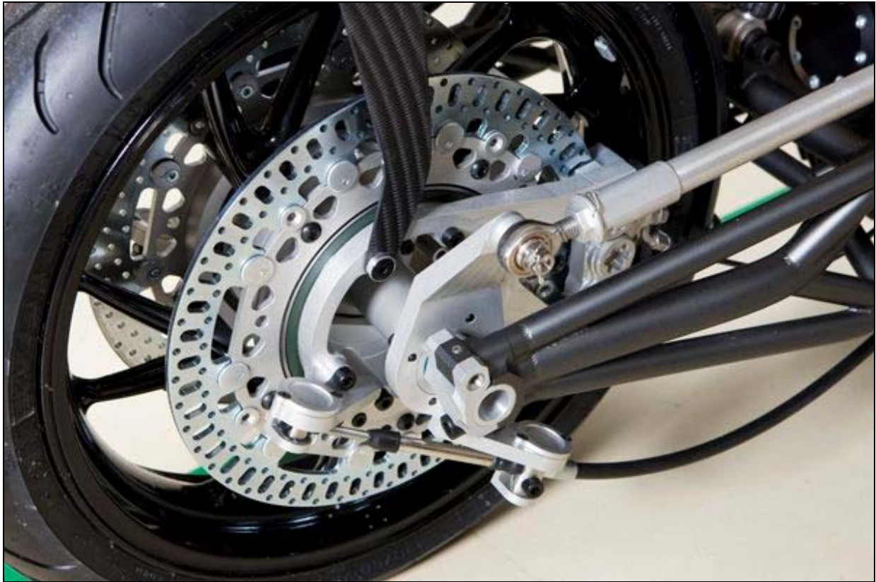
Figure 3.14. Stellan Egeland's custom BMW Harrier motorcycle front suspension with hub steering from ISR Brakes (Rising, 2010).
