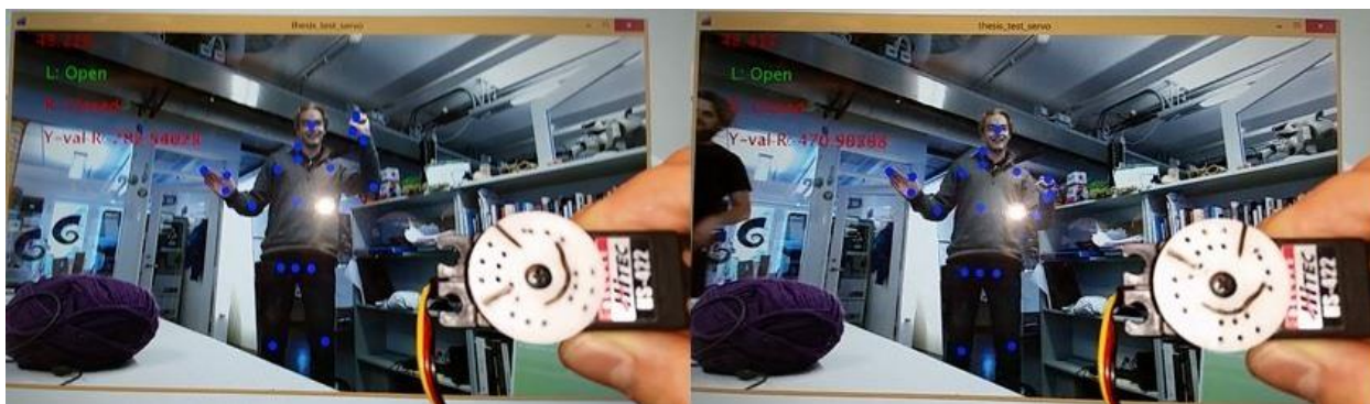
Figure 3.2. First successful implementation of control of a servo motor based on the location of a user’s hand.
