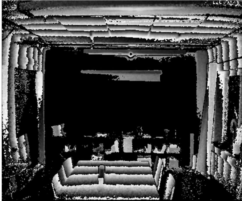
Figure 3.5. The signal from the depth camera transformed to greyscale with values 0 (black) to 255 (white).
