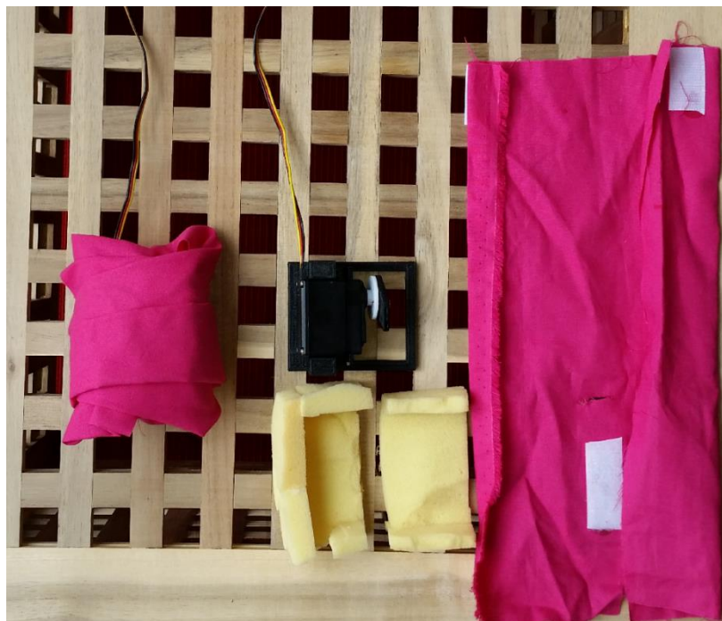
Figure 3.18: Prototype for investigation of different ways to map breathing. On the left an assembled prototype and in the middle the servo, its 3D-printed holder, and the Tempur used to create a soft feel.
