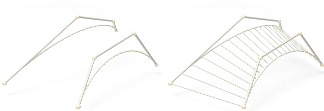
Figure 3.9: A ruled surface (right) could be represented and parametrized by connecting two curves (left). It is developable if and only if each ruling defines a common tangent plane shared by all its points.
