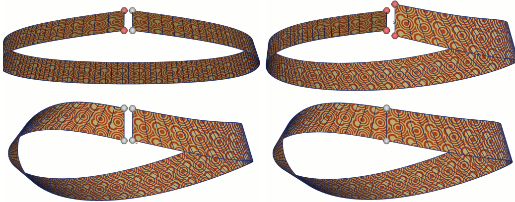
Figure 3.22: Isometric manipulation of a strip to create a Möbius band. The texture coordinates are interactively updated by the coordinates of the points on the development which is isometric to the spatial mesh and constrained on a given rectangle.
