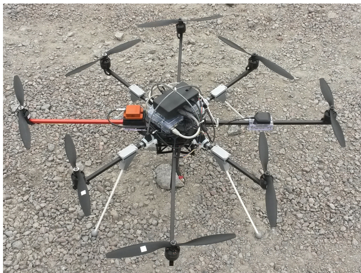
Figure 2.1: The new configured octocopter which is developed and used during the thesis. The upper black cases contains e.g., the Arduino Nano. The two Raspberry Pi's are contained in the two transparent cases. The red part on the left in the picture is the IMU, the GPS antenna is on the right.
