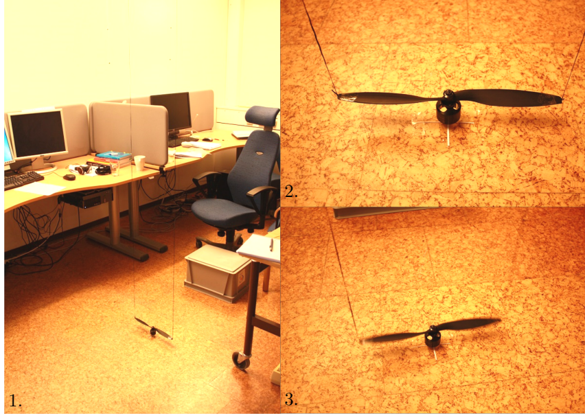
Figure 2.9: Experimental setup for motor and plastic propeller. 1. Hanging from the ceiling by two thin strings. 2. Completely at rest before rotation, cross underneath to mark stationary position. 3. Rotating about its vertical axis.
