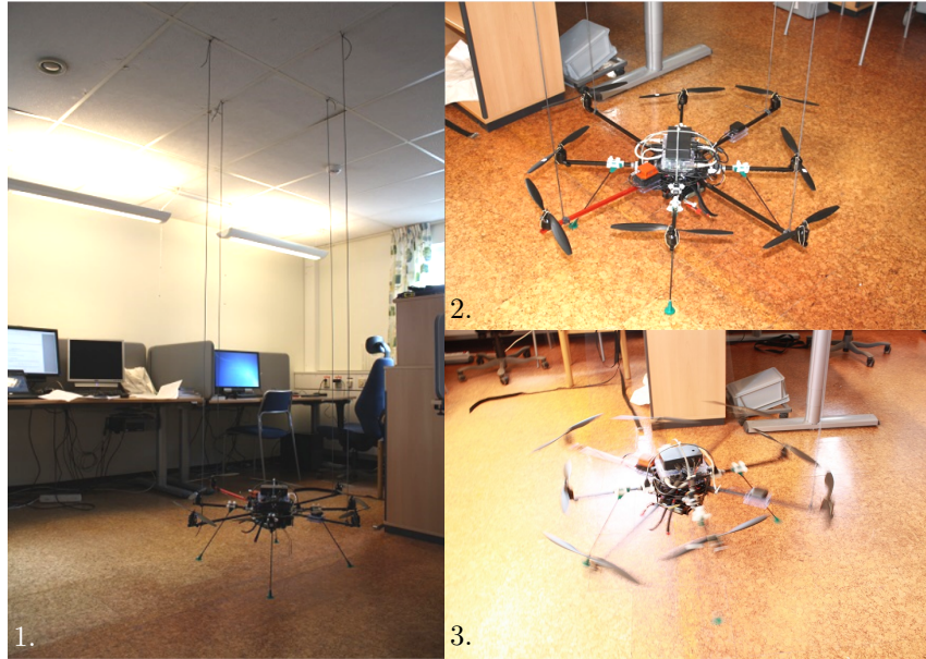
Figure 2.10: Experiment setup for octocopter. 1. Hanging from the ceiling by four strings. 2. Completely at rest before rotation. 3. Rotating about its vertical axis.
