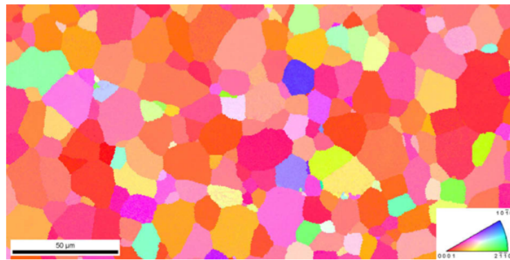
Figure 3.7: Example of EBSD orientation map showing the undeformed microstructure of a high purity clock-rolled Zr specimen. Colors designate crystal orientations as indicated by the unit triangle in the bottom right-hand corner. The software used to generate this map is OIM Analysis [93].
