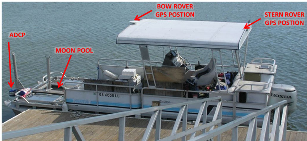
Figure 8: Image of docked field boat. Instrumentation identified.
