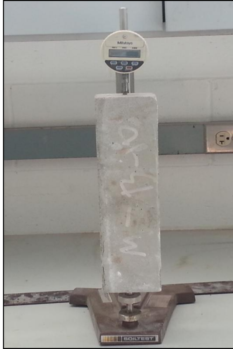
Figure 3.7: Unrestrained shrinkage test set-up and a mortar prism being tested.
