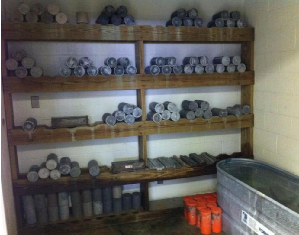
Figure 3.1: Concrete samples being cured in the curing room
