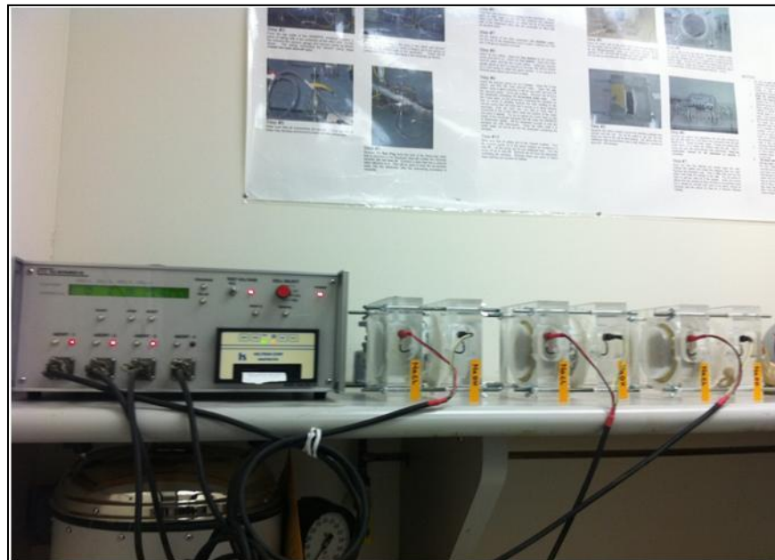
Figure 3.9: Rapid Chloride Permeability test set-up with all electrical wiring connected and test being performed.
