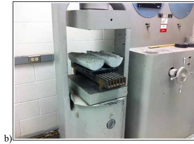
Figure 3.6: (a) Splitting tensile strength test set-up and (b) a typical failure mode of a concrete cylinder under tension.
