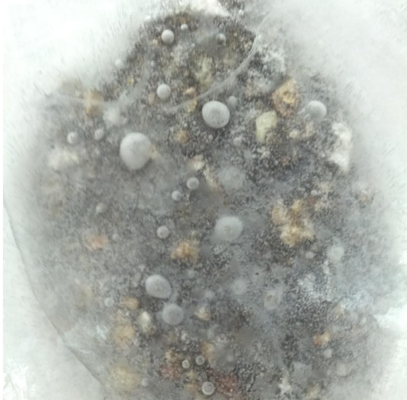
Figure 2.8: Iced asphalt sample: The spherical white-ish shapes are frozen trapped air bubbles, and the long sweeping lines (one of which can be seen on the bottom left section of the image) are fissures in the ice. Note there are sections of high and low clarity which occur naturally
