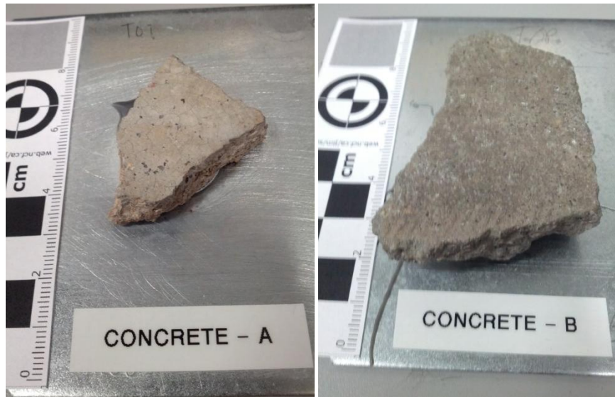
Figure 2.5: Concrete samples which have been mounted to steel plates using epoxy.
