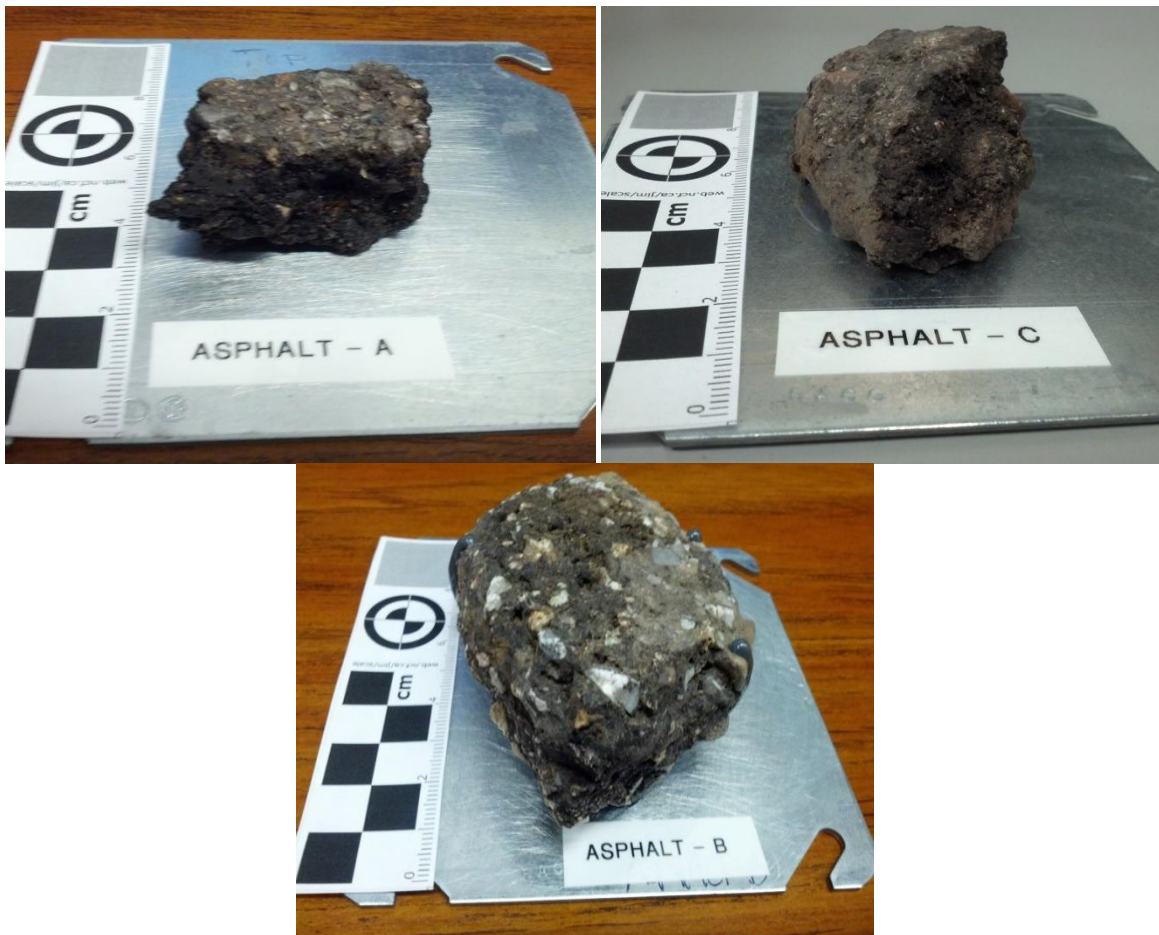
Figure 2.6: Asphalt samples which have been mounted to steel plates using epoxy.
