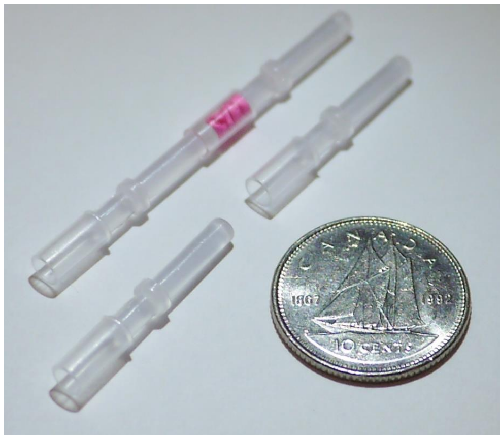
Figure 3-8 – The above image shows (from left to right) a connected VSM sample holder, a disconnected VSM sample holder, and a dime. The pink material in the connected sample holder illustrates how the sample would be contained in the VersaLab VSM.
