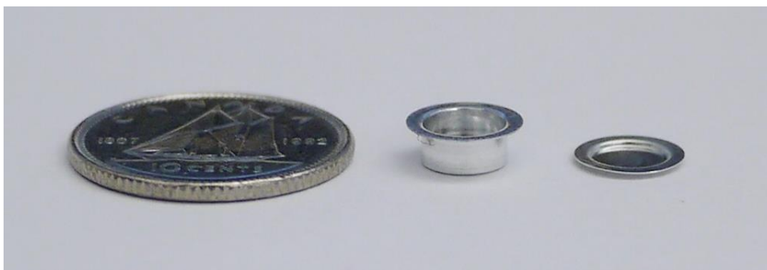
Figure 3-7 – From left to right the above image shows a dime, the mDSC sample holder, and the mDSC sample lid. The lid sits on top of the crucible in the orientation shown such that it reduces the volume of the crucible by a small amount.
