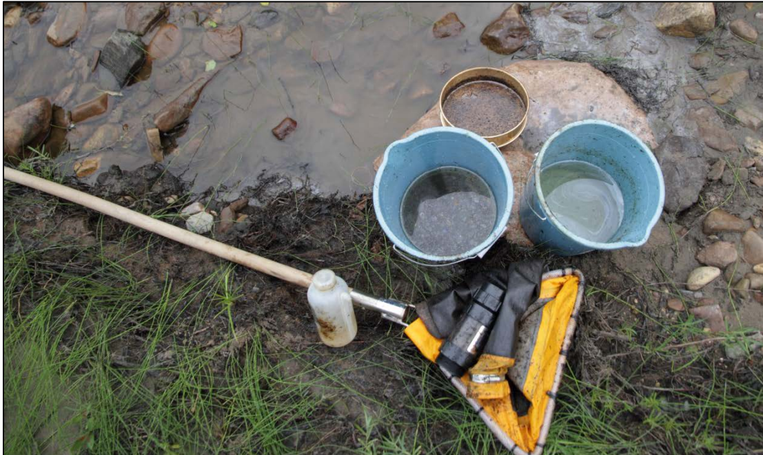
Figure 5.1. Equipment used for three-minute kick net, rock-basket retrieval and bulk kick net sampling for benthic macroinvertebrates at each site on the Steepbank and Ells Rivers during each sampling month (May-October 2012). Picture includes: d-framed 400 µm mesh kick net, 250 µm sieve, squeeze bottle and two buckets for elutriation procedure.
