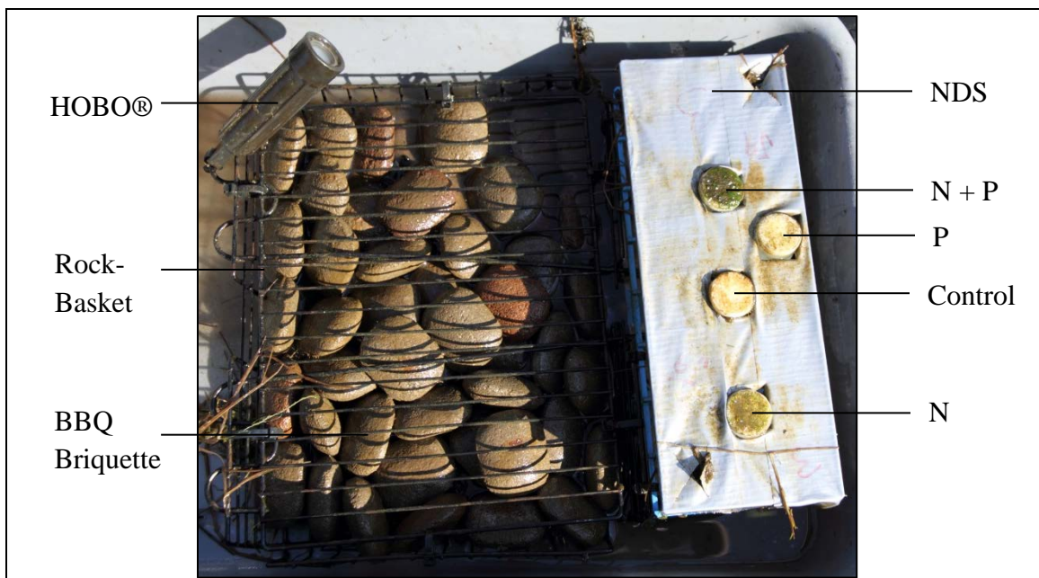
Figure 4.1. A retrieved nutrient diffusing substrata (NDS) fastened to a rock-basket artificial substrate containing 50 ceramic BBQ briquettes and a HOBO® data logger measuring water temperature ( ^{\circ}\text{C} ) every 30 minutes. Greatest periphyton growth was observed on the NDS treatment vial containing the nitrogen and phosphorus (N + P) agar mixture after the one-month deployment period in the example above.
