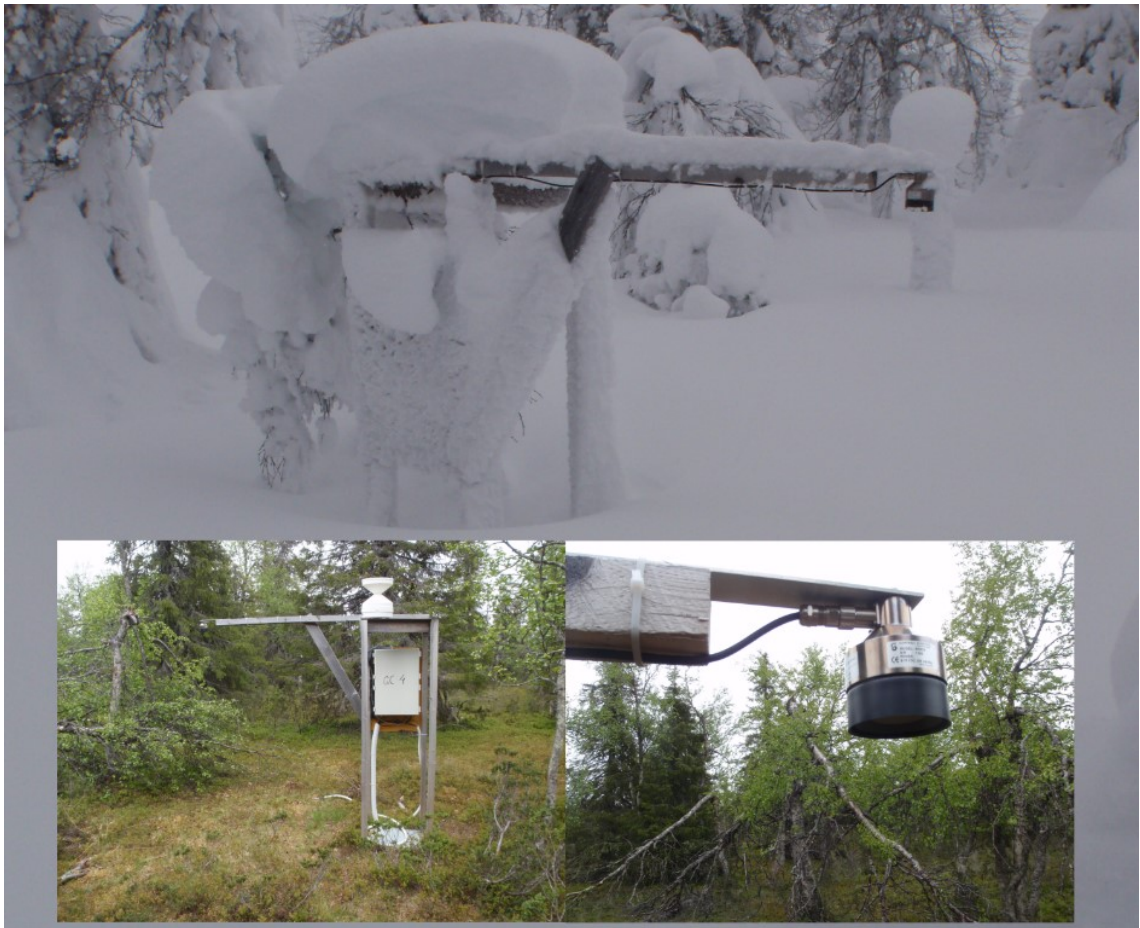
Figure 12. GTK measurement station GC7. SR50A SONIC RANGING SENSOR in small picture on the right.
