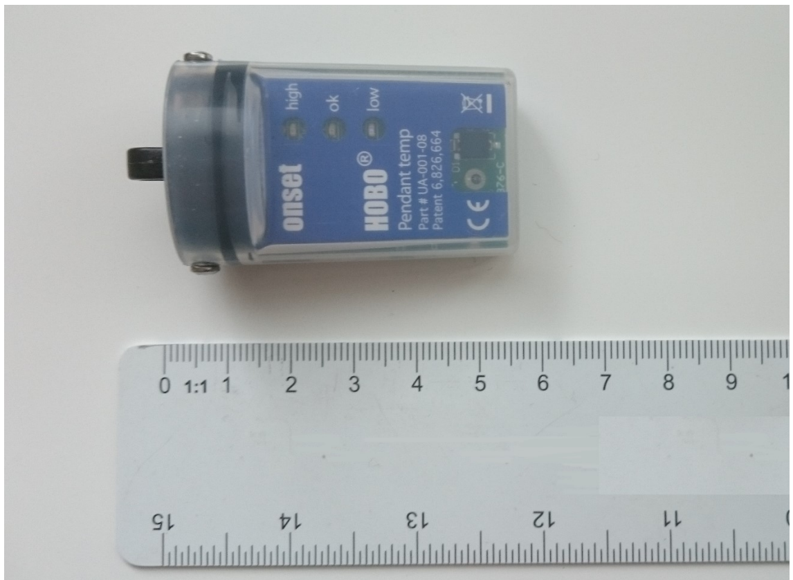
Figure 7. HOBO Pendant® Temperature/Alarm Data Logger 8K - UA-001-08.
