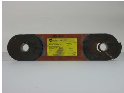
(a) Damaged specimen under fatigue loading conditions
