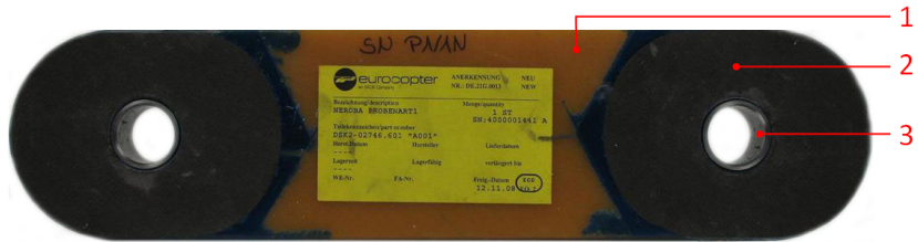
Figure 2.5: Lug specimen used for the NEROBA programme
