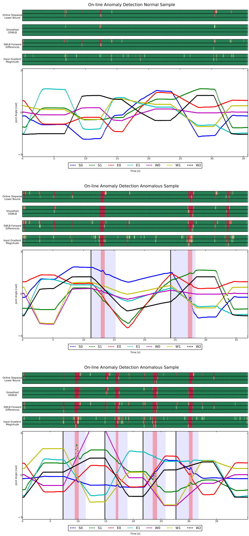
Figure 15: On-line detection for the unidirectional recognition model. The trajectories show one normal and two anomalous samples of joint configurations over time. The twelve bars on top show the four anomaly scores combined with the three thresholds \kappa_1, \kappa_2 and \kappa_3 . Green means that no anomaly is detected, red the opposite. Yellow colors indicate an anomaly score around the threshold.
