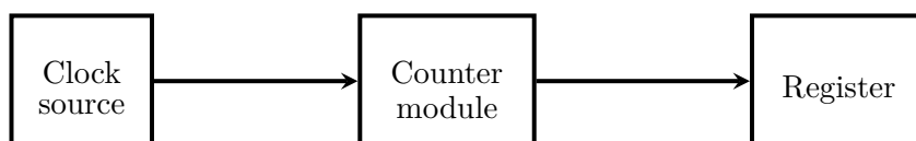
Figure A.2: A clock source, driving a counter, which increments the value in a register.
