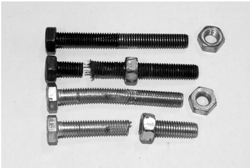
Figure 7.7: Bolts ruined in the process of locating the magnets with hose clamps.
