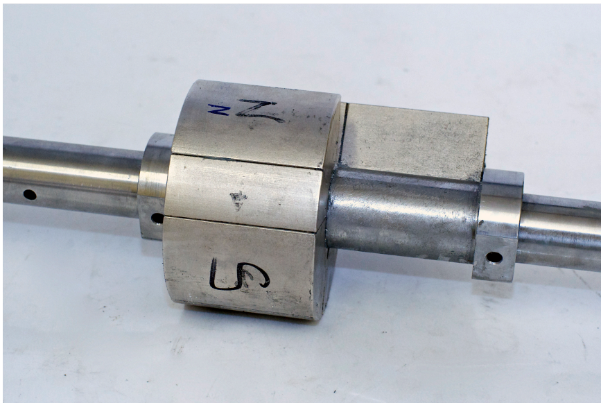
Figure 7.4: Process of fixing magnets in place with industrial adhesive.
