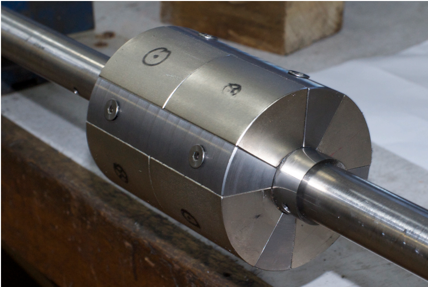
Figure 7.9: Completed translator with mild steel wedges replacing some of the magnets.
