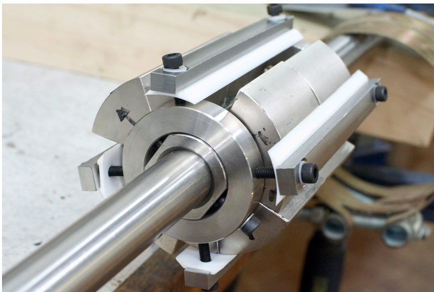
Figure 7.5: Radial magnet clamping technique in the attempted process of assembly.
