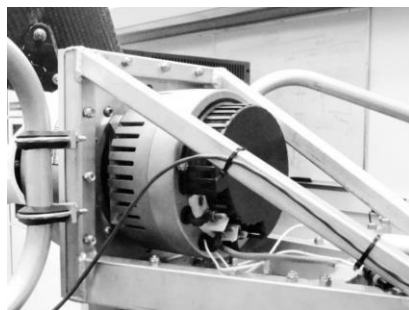
(a) PMAC motor/generator
