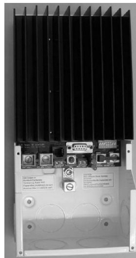
Figure 20. Dump load controller
