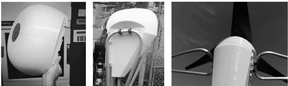
Figure 6. Custom 3D printed nacelle
