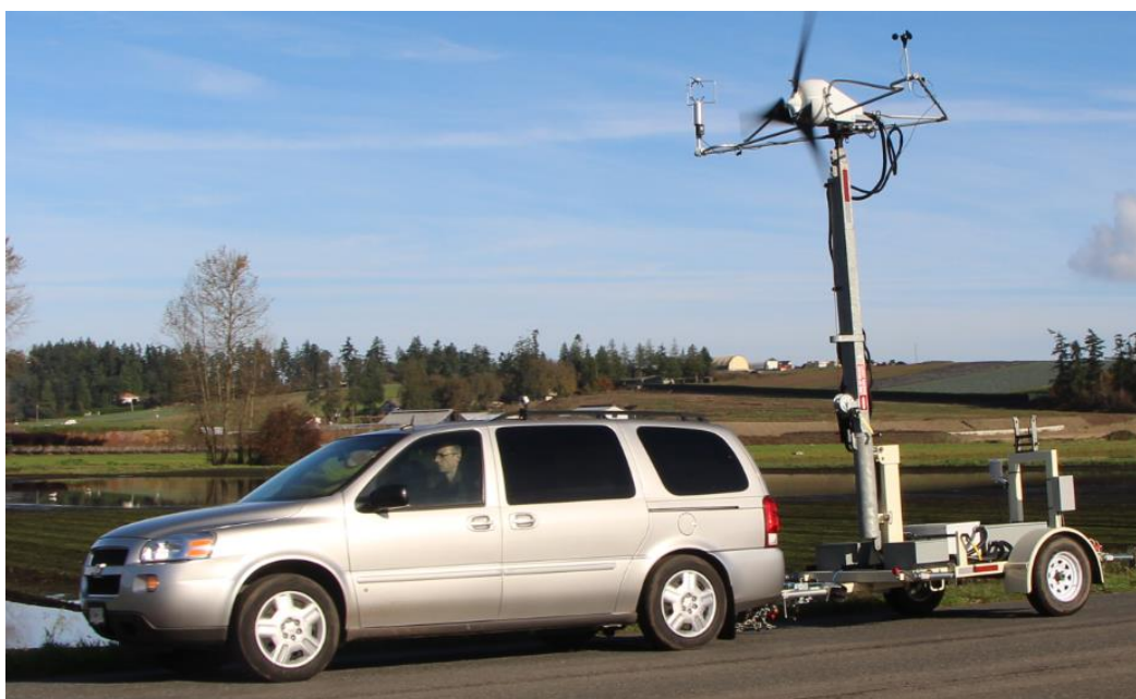
Figure 61. Controlled velocity track tests (towed scenario)
