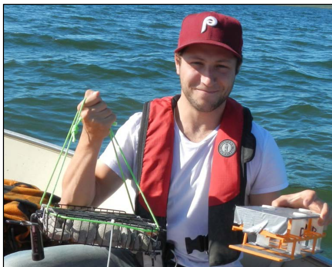
Figure 4-32: NDS (right) and briquette-filled barbecue basket (left) just prior to deployment in Noell Lake, NWT. Note the HOBOL logger on the left side of the basket.
