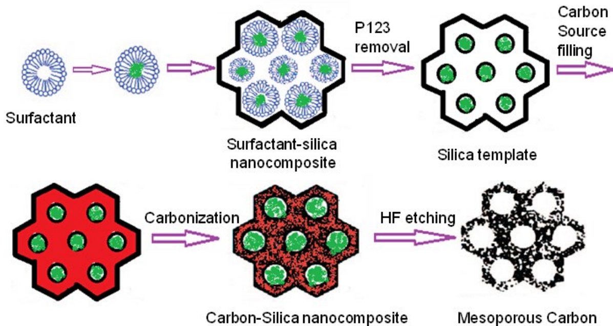
Fig. 5 Schematic illustration for the OMCs nano-casting strategy, viewing from perpendicular direction (100) (Lu Lin, 2011)
