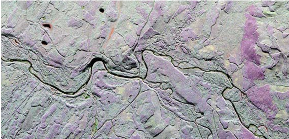
Figure 4 - PAULI decomposition of C-Band Polarimetric radar collected over Hinton Alberta with crescent shaped 50 year old fire scar visible on the right hand side of the image
