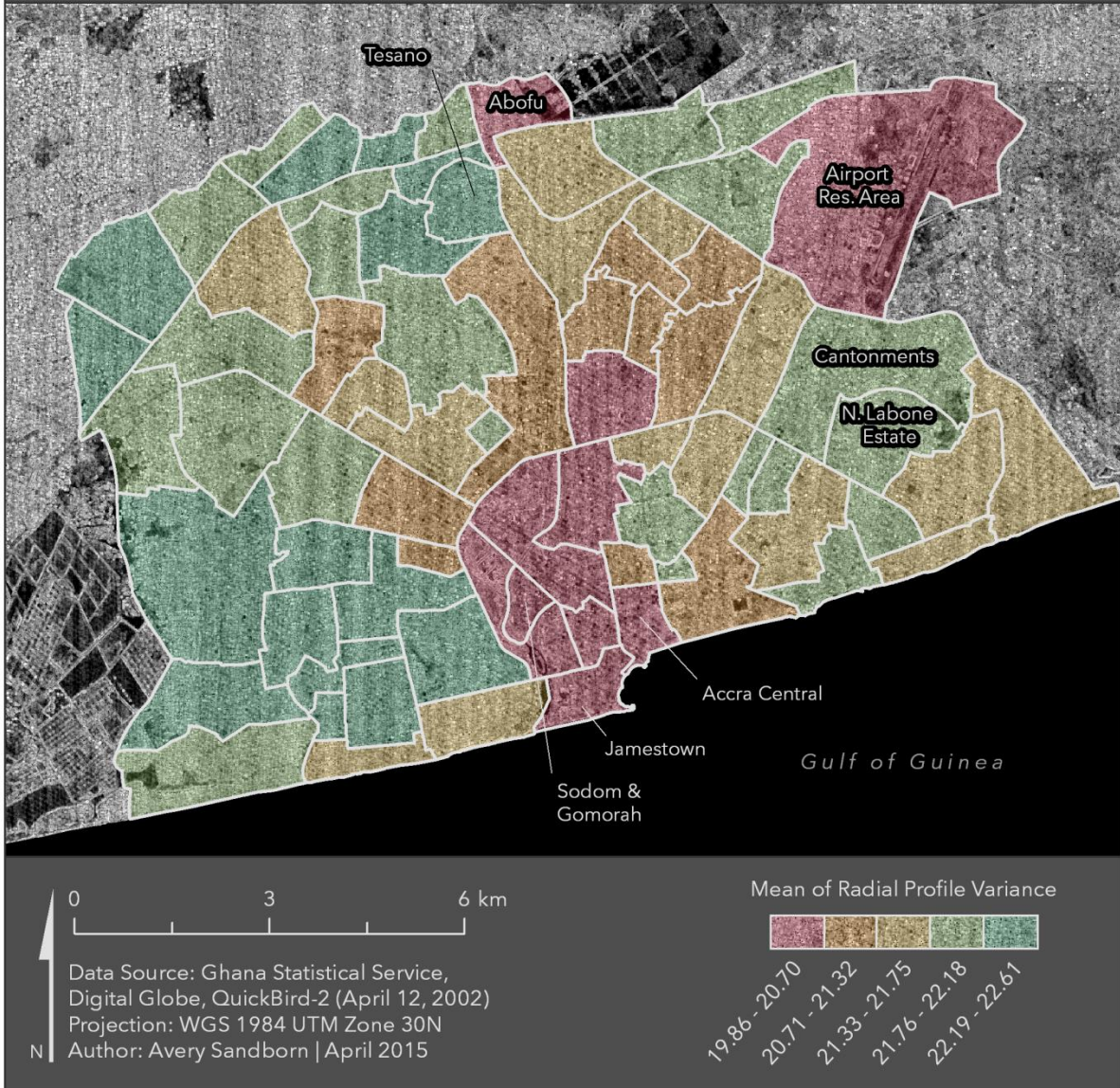
Figure 11: Fourier Transform (FT) Results: FT radial profile variance at block 4 and scale 16 is shown in this map. Higher values (shown in green) indicate a noisier power spectrum with many land cover variations, while lower values (shown in red) indicate a neighborhood with less land cover variations.
