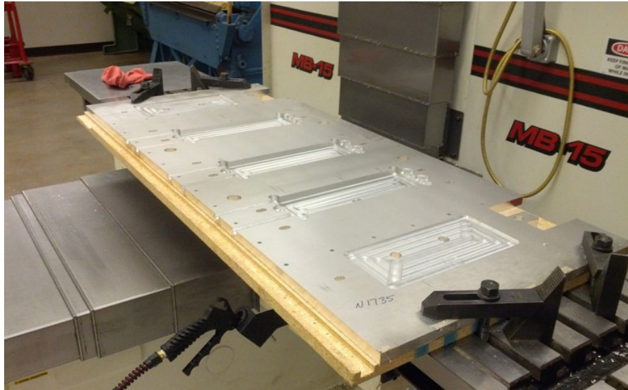
Figure 3.16. Middle aluminum Plate of the battery box - post CNC fabrication.
