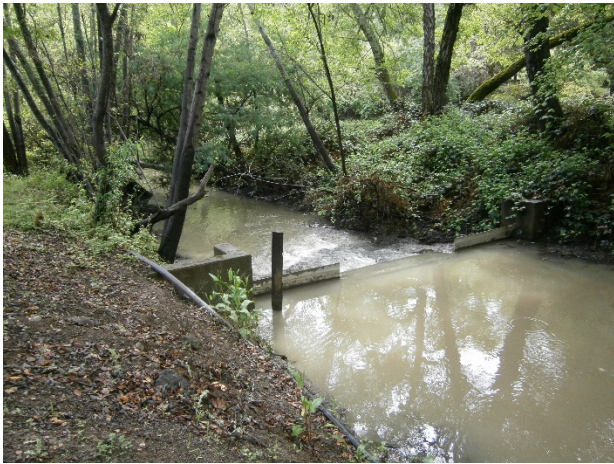
b. SCVWD Streamflow Gauge SF84 located approximately 30 m downstream of Uvas Reservoir Outlet.
