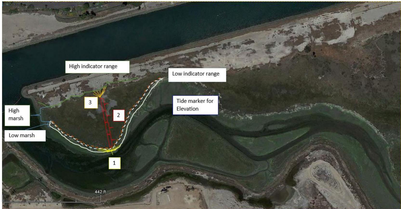
FIGURE 12. 1) The low marsh elevation is determined here after referencing the location of the sea level. 2) Elevation surveys begin at the upper extent of the high marsh and are used to determine the elevation change throughout the marsh plain. 3) Continuing from the first occurrence of the marsh plain, several elevation points are collected to determine the high marsh extent.
