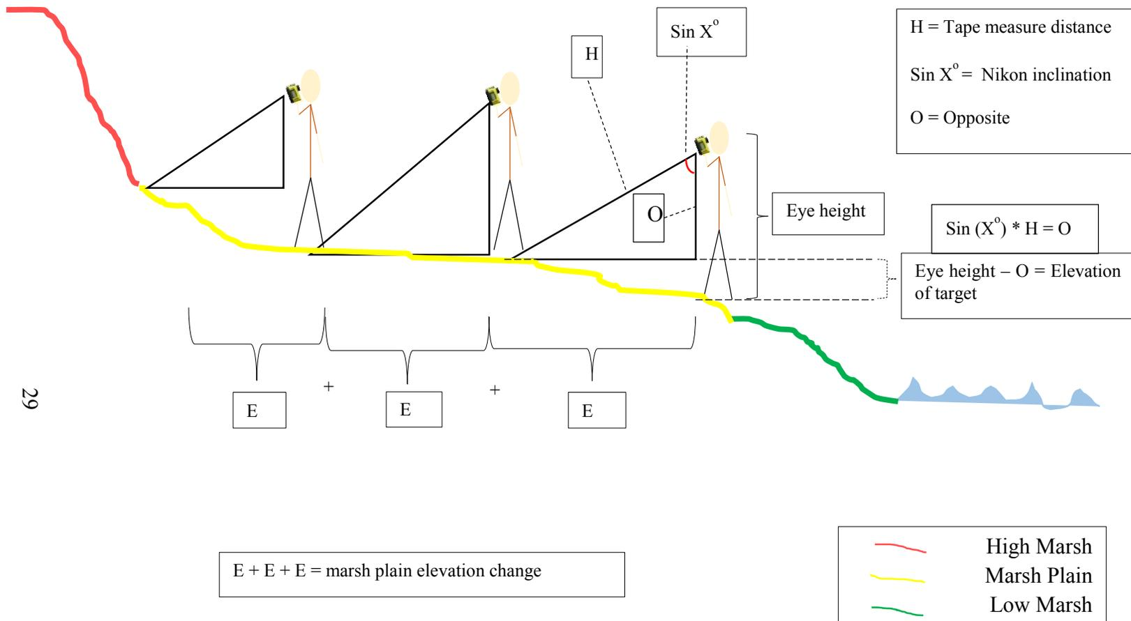
FIGURE 10. The illustration helps visualize the elements of the sine equation used in elevation measurements. The animated researcher aims the Nikon at the ground to determine elevation change. All of the elements in the sine equation are illustrated beside the researcher on the far right. The chain of elevation measurements, marked as E, determines the overall elevation change along the marsh, with the elevation measurement on the far left targeting an indicator species.
