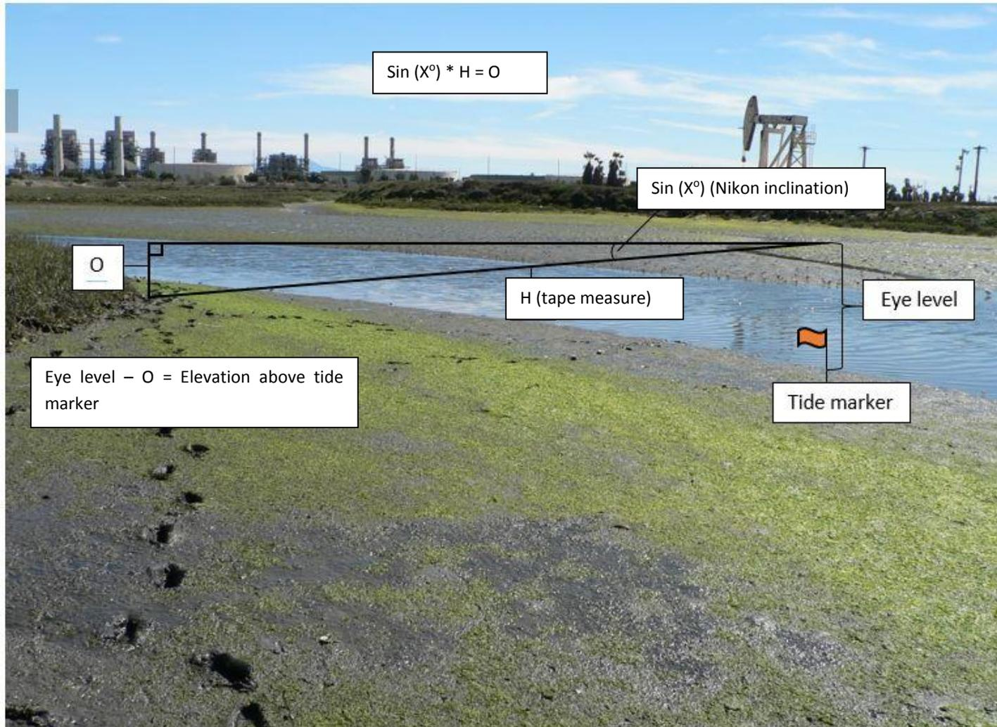
FIGURE 11. This illustration provides a reference for the elements of the trigonometry equation at a location where a survey was performed.
