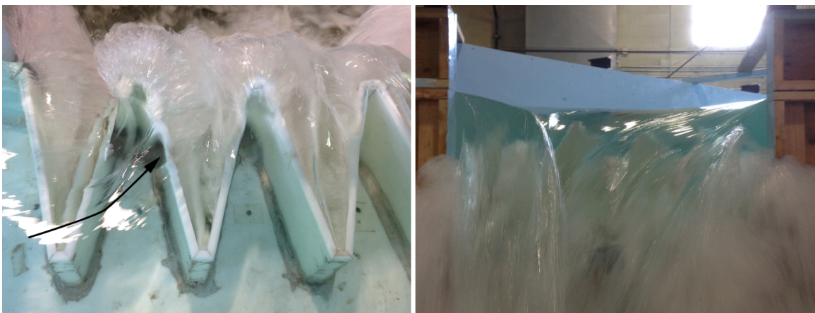
Fig. 33. Flow conditions for \beta = 45^\circ , showing imbalance at (a) H_t/P = 0.5 and (b) H_t/P = 1.0
