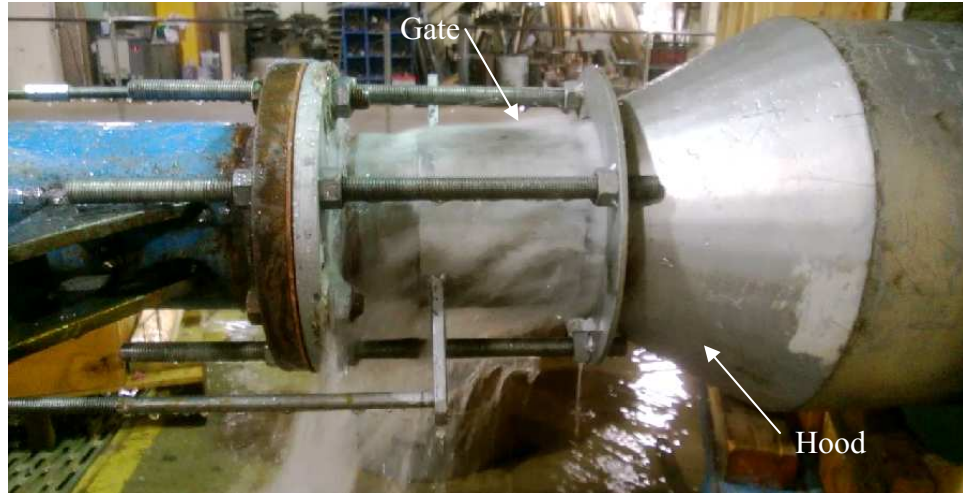
Fig. 2. Backslash occurring with a hooded-FCV.
