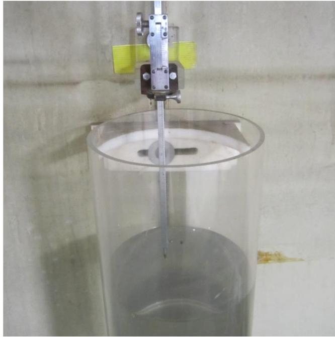
**Fig. 11.** Stilling basin with point gage
