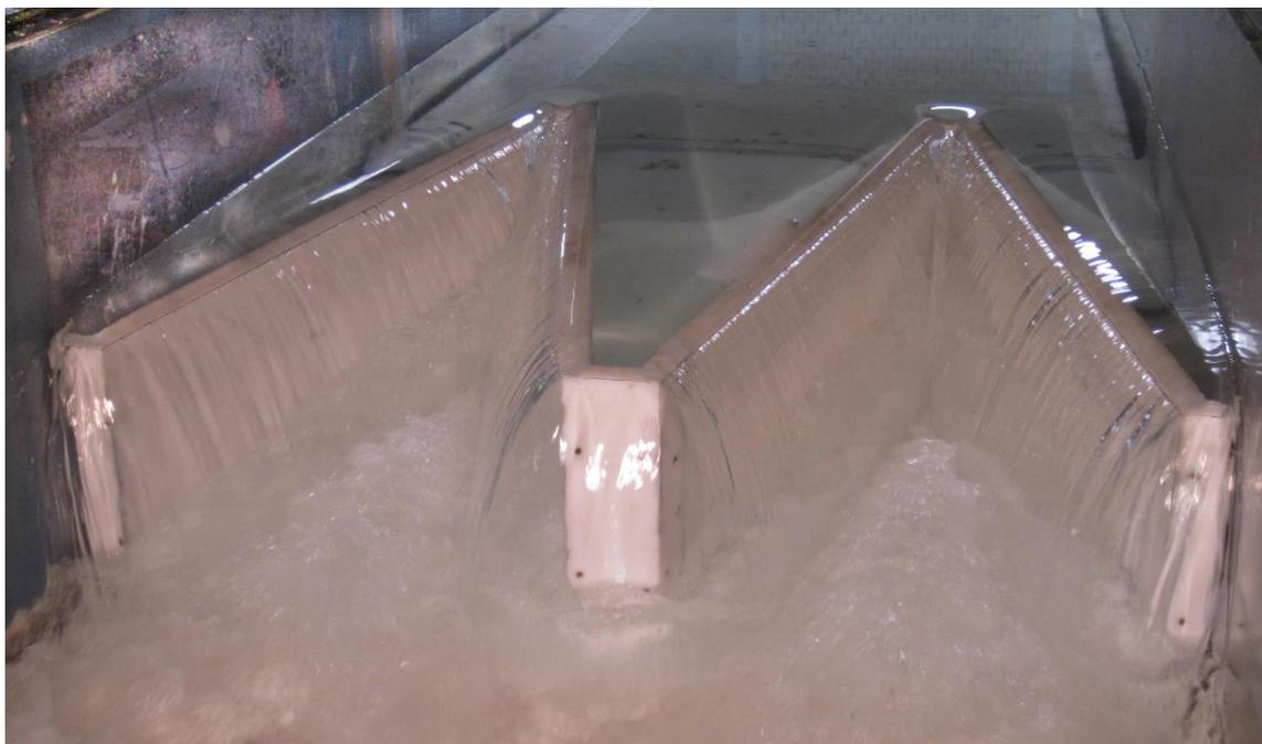
**Fig. A-12.**  $\alpha = 12^\circ$ ,  $QR$ ,  $A=1t_w$ , inverted orientation,  $H_T/P = 0.1$ , photograph
