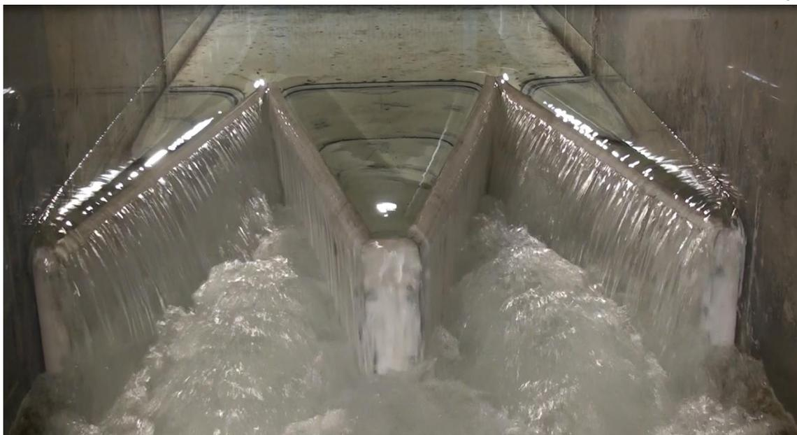
**Fig. A-5.**  $\alpha = 12^\circ$ ,  $HR$ ,  $A=0t_{w-us}$ , inverted orientation,  $H_T/P = 0.147$ , photograph
