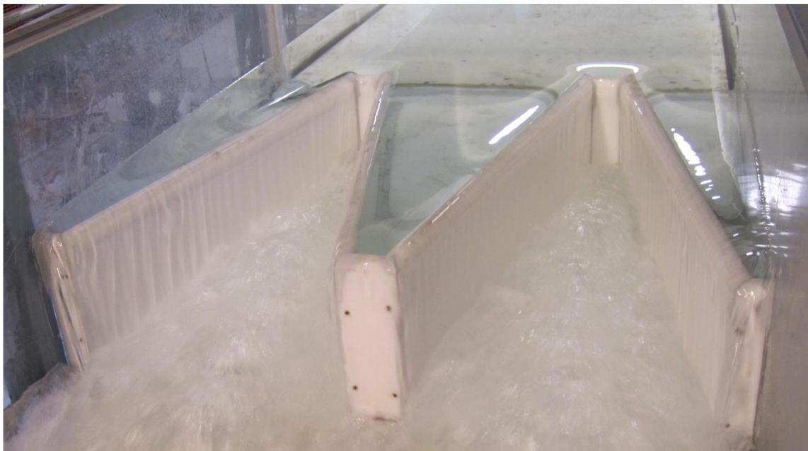
**Fig. A-14.**  $\alpha = 12^\circ$ ,  $HR$ ,  $A=2t_w$ , inverted orientation,  $H_T/P = 0.1$ , photograph
