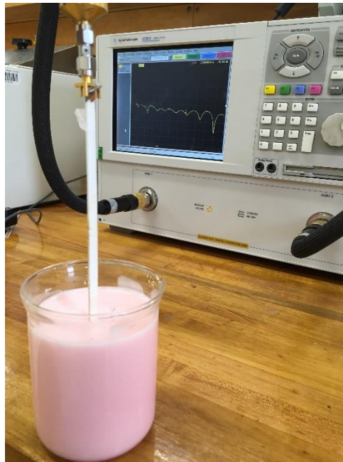
Figure 3.2 Ultra-wideband applicator encased in liver mimicking gel
