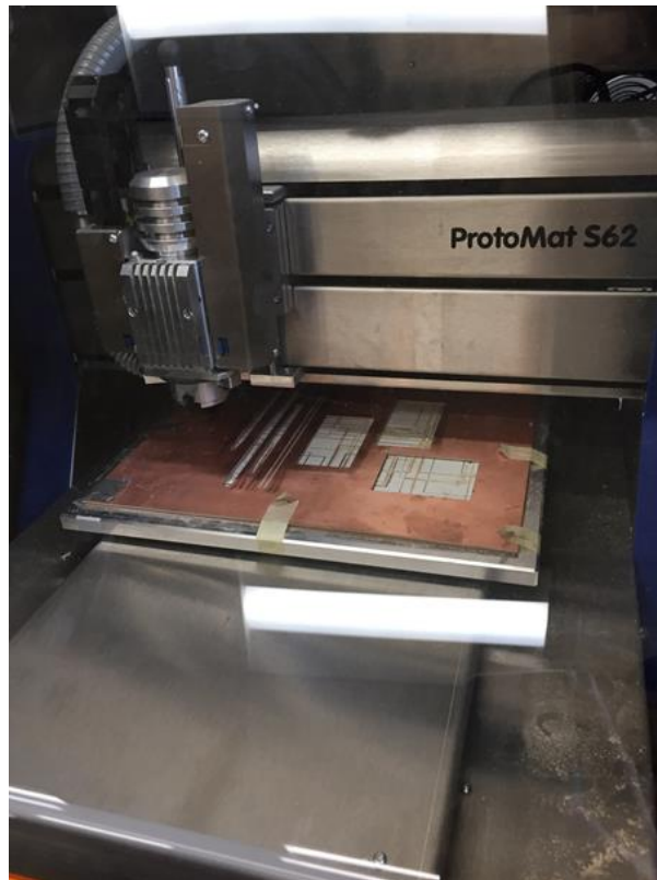
Figure 2.22 Antenna applicator fabrication process
