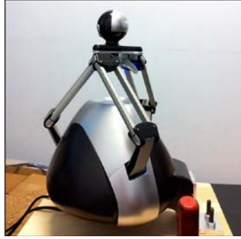
FIGURE 2. Screenshot of the Novint Falcon force feedback device.
