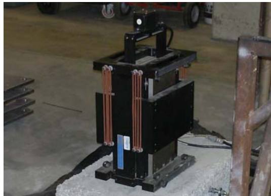
FIGURE 3.5. (From Star 2011) Picture of Atom Ant used for loading of SSI test structure.
