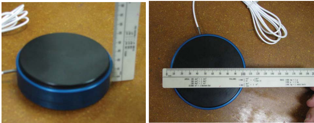
FIGURE 3.8. Pressure cells similar to those used in UCLA field test (Photo: A. Lemnitzer).
