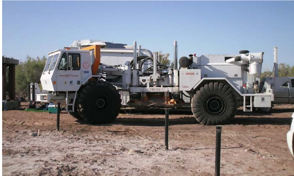
FIGURE 3.7. (From Star 2011) Tri-axial vibroseis shaker truck.
