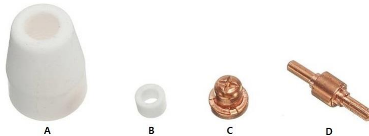
FIGURE 10. PT-31 torch head components. A: Shielding cap, B: Flow swirler, C: Nozzle, D: Cathode. Shielding cap holds all the components in place. Flow swirler changes an incoming axial flow to a vortex flow. Nozzle constricts the flow. Cathode is a terminal that produces electrons.
