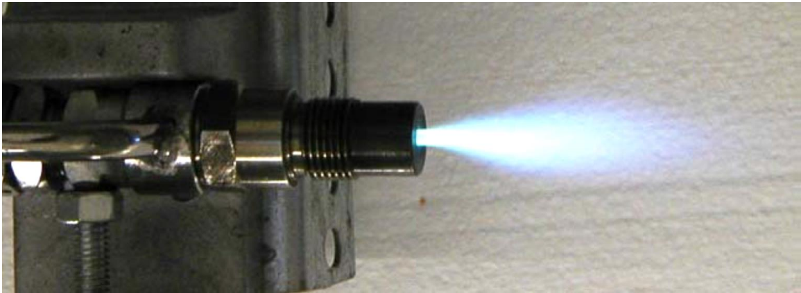
FIGURE 1. Combined cycle plasma torch in operation [11].
