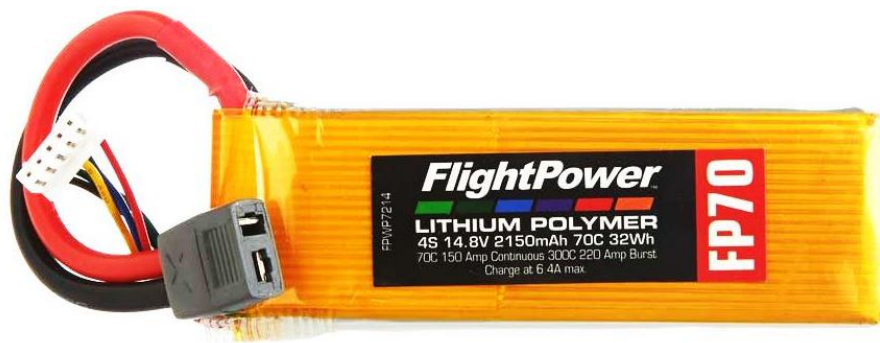
FIGURE 30. FlightPower lithium polymer battery (FP70 4S 2150mAh). Output voltage: 14.8V, capacity: 2150mAh and C-rate for continuous discharge: 70C (150.5A).
