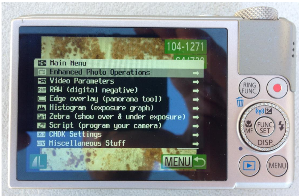
FIGURE 17. Canon S110 camera running CHDK hack.
