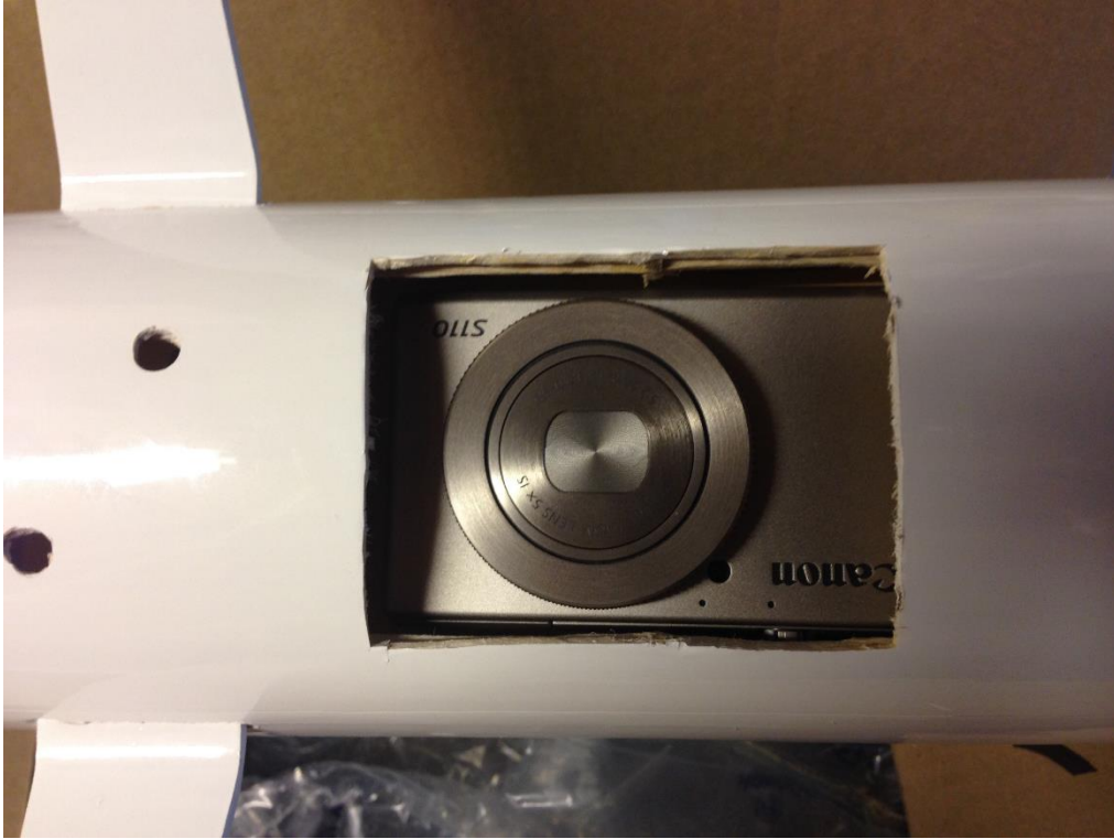
FIGURE 10. Camera installation in the nadir position.
