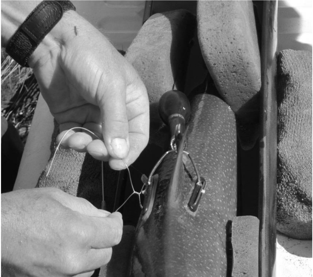
Fig. 1.3. X-tag attached to a Dolly Varden with a wire harness “tag backpack” attachment system.
