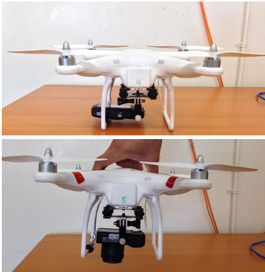
FIGURE 8. PENTAX Optio WG-II GPS mount (top) and Ricoh GR III mount (bottom).
