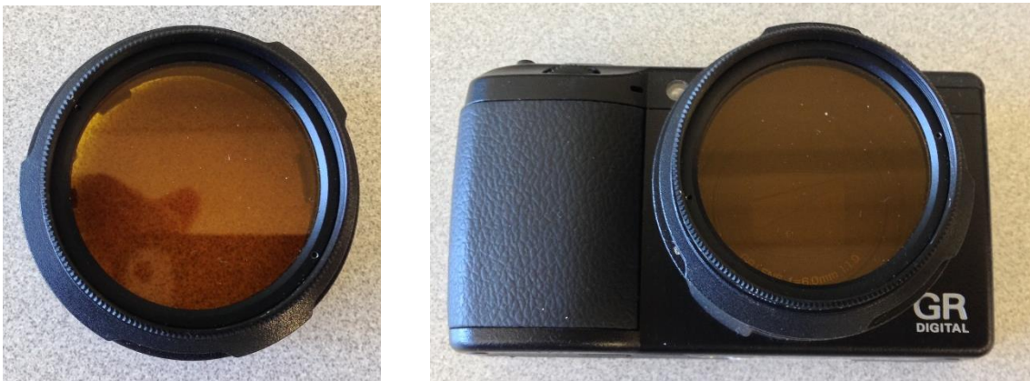
FIGURE 6. Tiffen 43DY15 43mm deep yellow 15 filter (left). It was outfitted on the Ricoh GR III (right).
