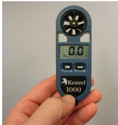
Figure 30 Kestrel 100 wind meter
