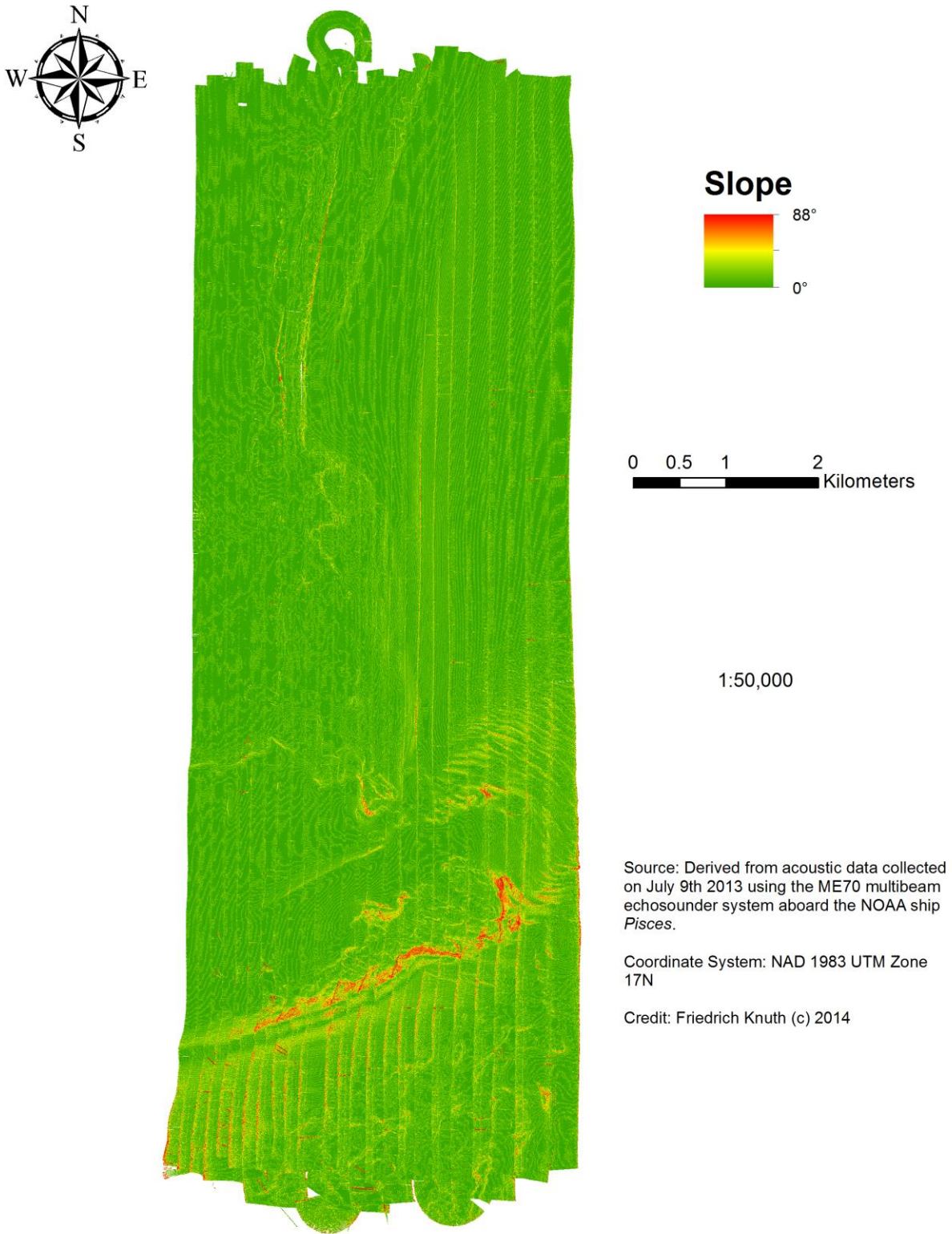
Figure 39. Maximum rate of change in depth between 2 x 2 m raster cell and eight neighbors at Bull's Scarp.
