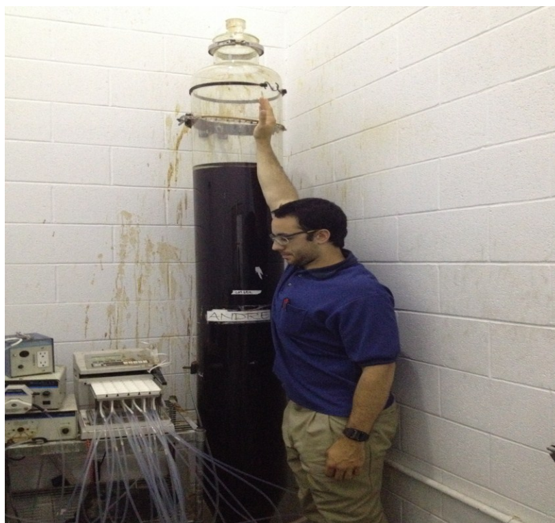
Picture 3. 8" x 96" C18 Column with a large scale fraction collector
