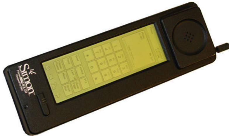
Figure 2.3: The IBM Simon released in 1993. The World's first smartphone. (Courtesy of WonderHowTo)
