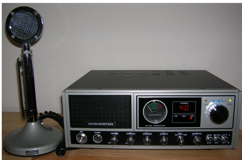
Figure 3.1: CB Radio Base Station
