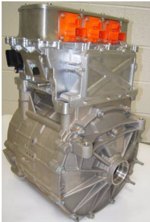
Figure 2.8: Magna E-Drive - Integrated inverter, motor, and differential (Image courtesy of UVic EcoCAR2 Team)
