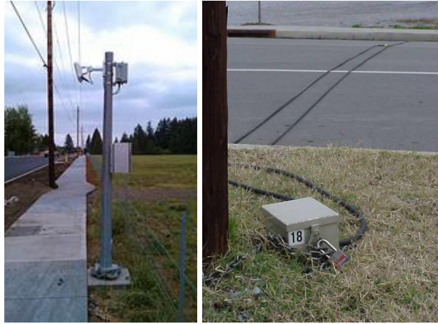
Figure 1: Permanent (Left) and Portable Temporary (Right) Traffic Counting Devices Images Courtesy of: Flickr Profile Rob Klug (Left) and City of Knoxville, Tennessee Traffic Engineering Division (Right)
