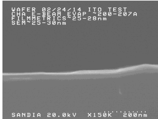
Figure 3.3: SEM image of ITO on reference substrate confirming thickness of ITO using E-beam deposition
