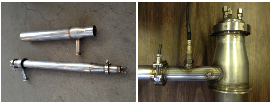
Figure 3.5: Steam reformer and heat exchanger shell (L), and top detail (R)
