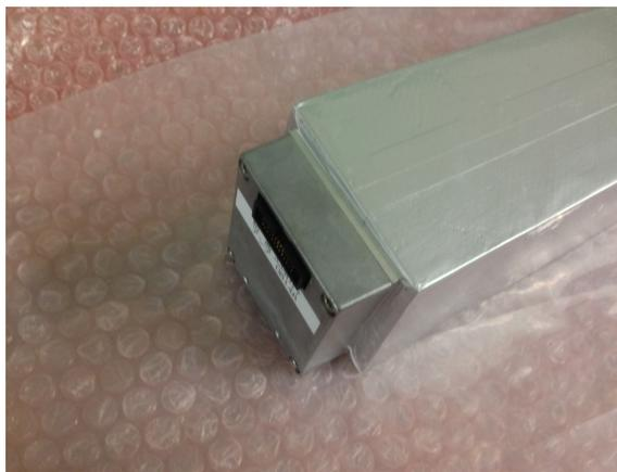
Figure 4.7: Preamp assembly at back of Belle crystals.
